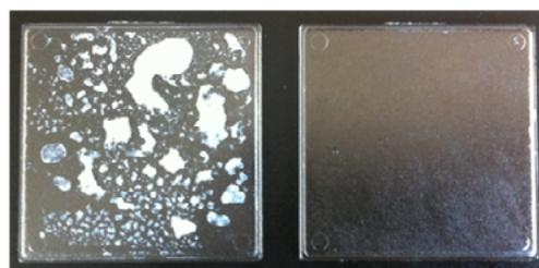
Figure 2: Comparison of spray residuals on wet substrate (sunscreen products leave white marks on the left plate, transparent film on the right plate)
